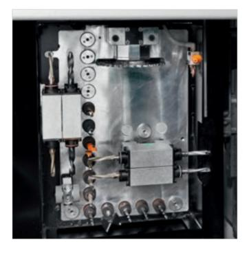
11 kW electrospindle equipped with an HSK F63 snap-on coupling to perform any machining operation using tools and aggregates.
