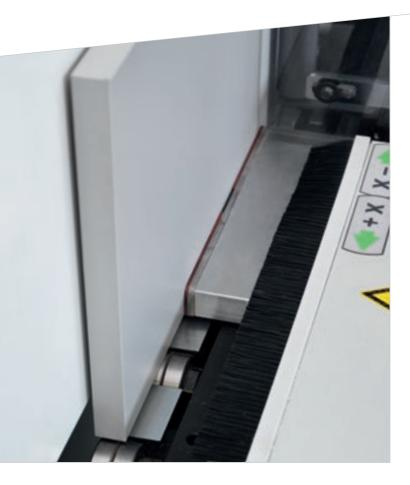
Brema Eko 1.1 is the ideal solution for "just-in-time" production: set-up time is equal to zero, as the panel is handled by a fully automatic clamp.
