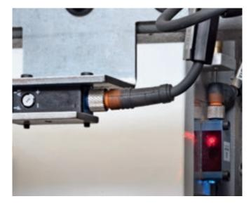
The laser scanner system that detects the start, end and height of the panel means that the machine can offset dimensional errors, by correcting the "X" and "Y" dimensions of the machining operation.
