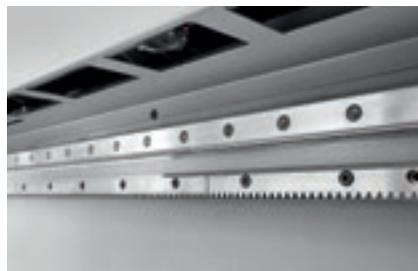
Oversized rack guides and pinions for movements on the X and Y axes, to obtain the maximum speed and acceleration in this category. Machine stability during movements is enhanced, thereby increasing the level of machining precision and quality.
